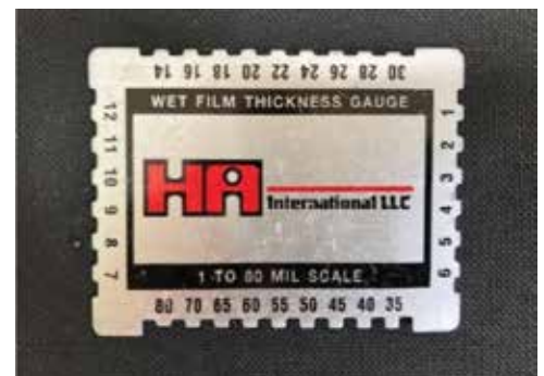
Figure 6: Wet Mil Thickness
